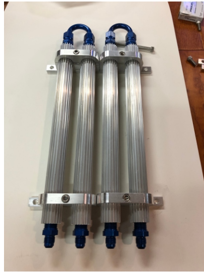
Reassemble as shown above on the four tube mounting bracket. The blocks are factory installed approximately 7/8" from the end of the finned tube. Do not torque down allen bolts yet. It maybe necessary to slide one tube assembly to align the two center tubes to install the 180 degree fitting. This is important so you can have all fittings relaxed to achieve the proper seal of your assembly.
