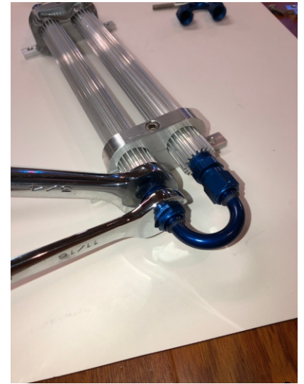
Always tighten fittings as shown above using 11/16" and 3/4" open end wrenches.
