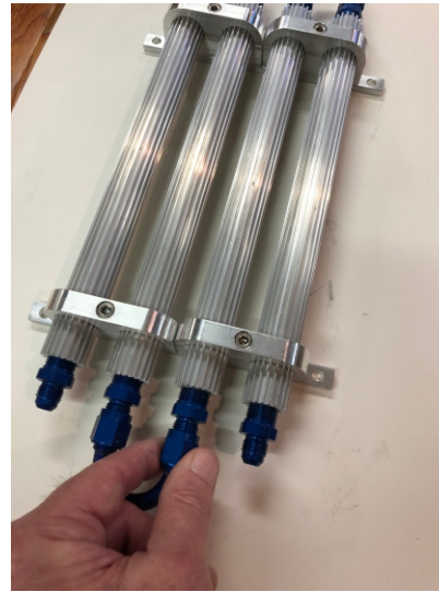
Install the 180 degree fitting turning both nuts at the same time to properly seat the fittings. You will feel the fittings seat and should rotate freely as you rotate them into place. Tighten by finger only, no wrenches. After getting fittings as tight as possible by hand you can now tighten the bolts securing the blocks and tubes to the mounting brackets. The blocks should be 7/8" from the end of the finned tube.
